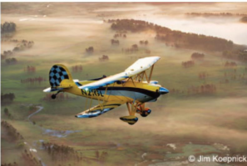
A 180 hp Lycoming IO-360 powers the biplane, which climbs at 1,400 fpm and cruises at 105 knots.
